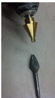
Drill lid slowly and carefully reversing sides, use rasp to finish hole smoothly, insert plug, needle, gauze.
