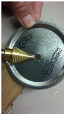
Drill lid slowly and carefully reversing sides, use rasp to finish hole smoothly, insert plug, needle, gauze.
